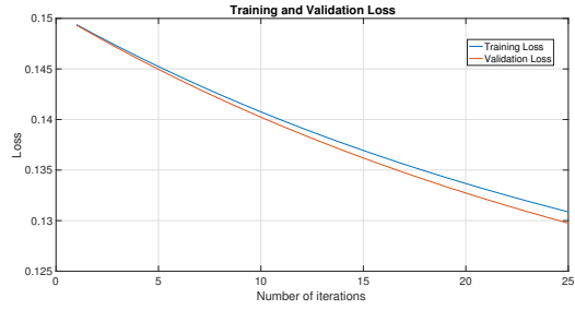
Figures 6-7: Training and validation performance of Algorithm 1.3 on the 1-layer ELM: (Left) Accuracy stabilizes across iterations, (Right) Loss decreases, indicating effective learning and convergence.
